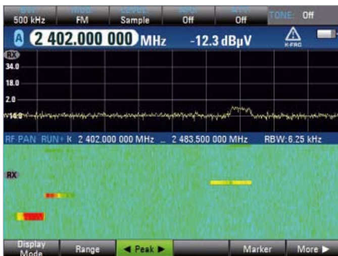
Bluetooth® hopping signals: Europe + US band: 2.402 MHz to 2483.5 MHz.
