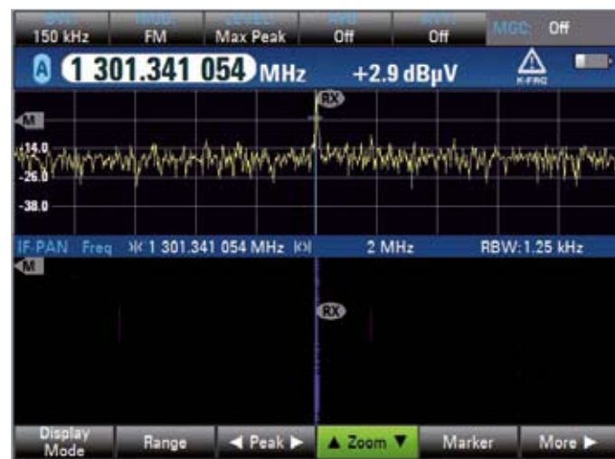
433 MHz ISM non-licensed band TX signal: garage door opener; 2nd harmonics.
