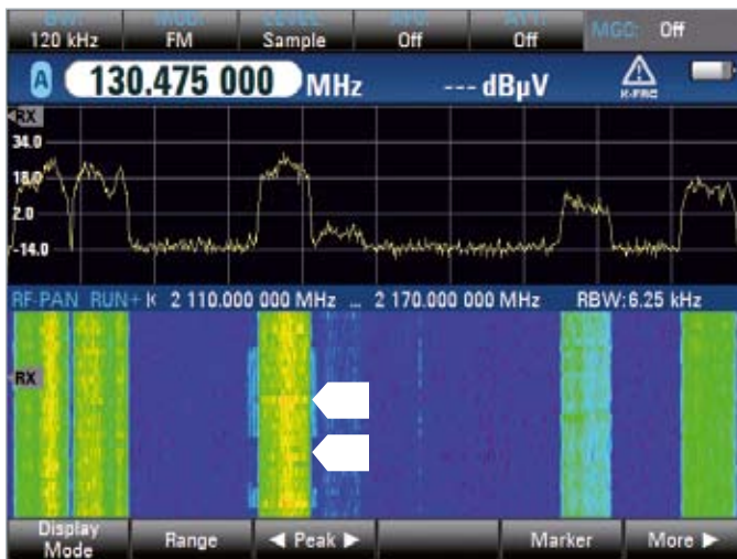
WCDMA TX bandwidth problem in WCDMA downlink band: defective amplifier and/or faulty duplex filter and/or intermodulating antenna system.
